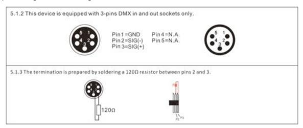
5.1.4 Connection: us DMX cable with 5 pin XLR-plugs to connect the controller with the fixture or one fixture with another.
