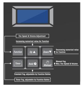
**FUNCTION:**Function switching button; then have the numerical value changed by using UP and DOWN buttons.
