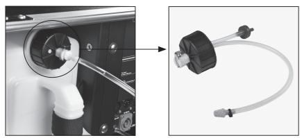
**2.** Prolonged use, the nozzle may be clogging by impurities, periodically use tools to clean the nozzles, keep the nozzle unobstructed.
