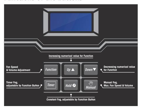
**FUNCTION:**Function switching button; then have the numerical value changed by using UP and DOWN buttons.
