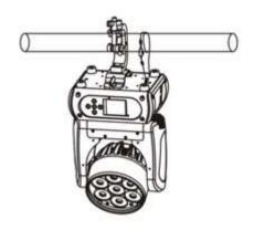
Step one: Installation the clamp onto the omega bracket;
