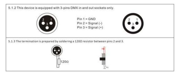
5.1.4 Connection: us DMX cable with 3-pin XLR-plugs to connect the controller with the fixture or one fixture with another.
