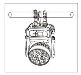
Step two: Install the clamp and bracket on the bottom of panel, fasten the quick-locks;
