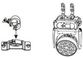
Step one: Installation the clamp onto the omega bracket;
