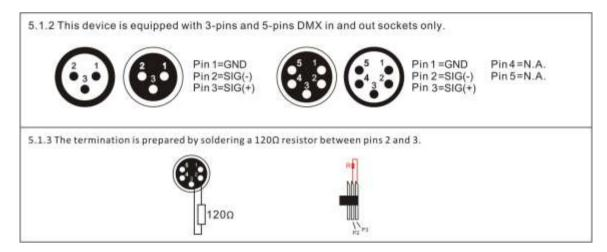
5.1.4 Connection: use DMX cable with 3+5 pin XLR-plugs to connect the controller with the fixture or one fixture with another.
