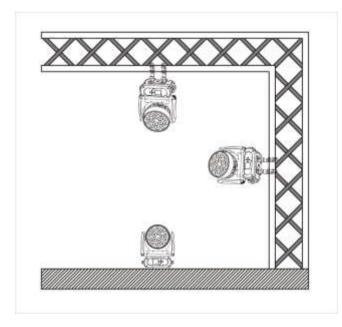
3.1 The device could be either put on a solid and even surface, or mounted upside down or sideways like left picture.
