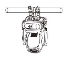
Step one: Installation the clamp onto the omega bracket;
